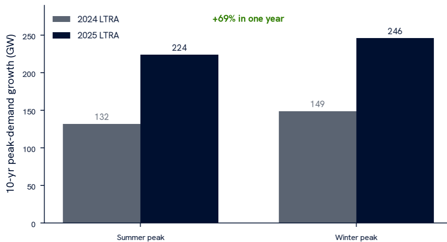
Figure 4. Ten-year peak-demand growth as projected by NERC's 2024 and 2025 Long-Term Reliability Assessments. The one-year jump — roughly 69% for the summer peak — reflects data-center load, electrification, and manufacturing, and is the steepest revision in decades.
